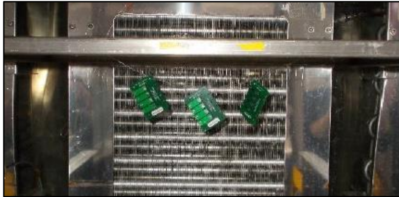
Samples in Salt Spray Chamber
