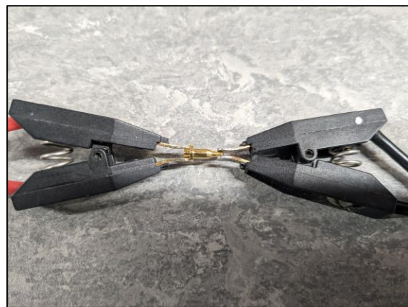
Fig 4: Contact Resistance (Loose samples) Test Set Up.
