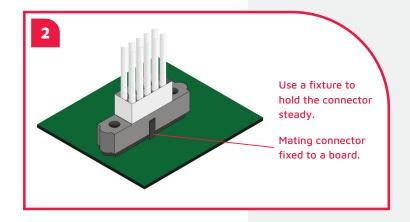
The simplest fixture is to glue a mating connector to a rigid board, and mate the connector being potted. Alternatively the connector could be held in a small vice – it is recommended that the connector is still mated in this method.
