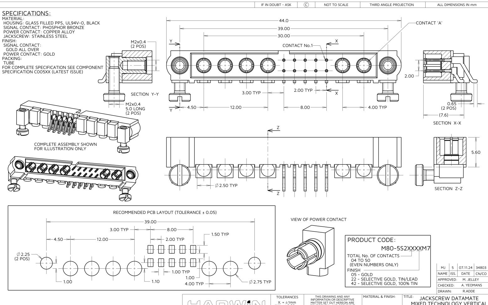
1. CONNECTORS ARE SUPPLIED WITH SCREWS LOOSE.
