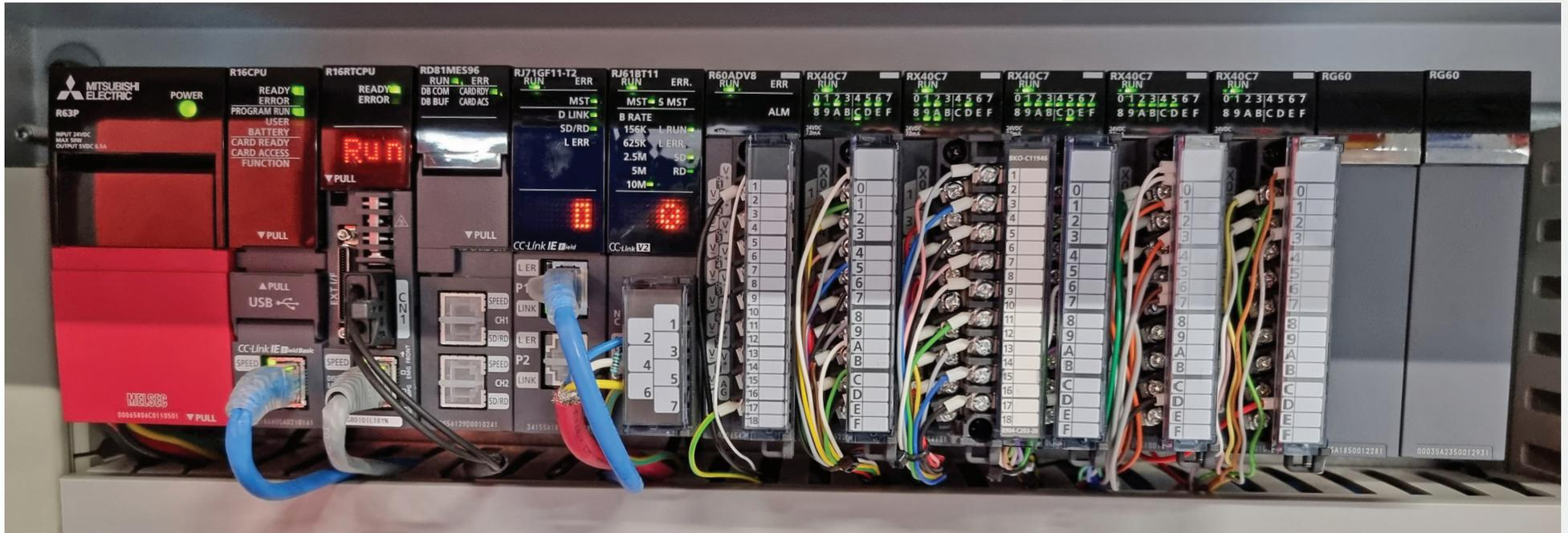
*Automation on the Harwin assembly line: Power supply, PLC, communications and input modules*
