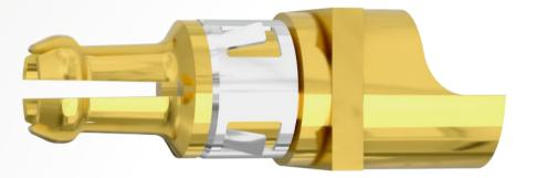
In contrast to the other HRi high-reliability connectors (where the female contact is the heart), here you'll find a 6-fingered Beryllium Copper male contact providing a positive normal spring force against the female mating contact. The durable hard-acid gold finish ensures repeated mating cycles and long-term environmental exposure do not affect the connection surfaces.
