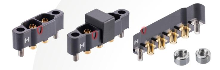
For the <u>male board connectors</u>, these are also available in 2, 3 and 4-contact single row options for PCB throughboard mounting in vertical, with 4.5mm or 5.9mm PC tail terminations. They also display a contact no. 1 marker, and are supplied in tubes with pick and place caps fitted.
