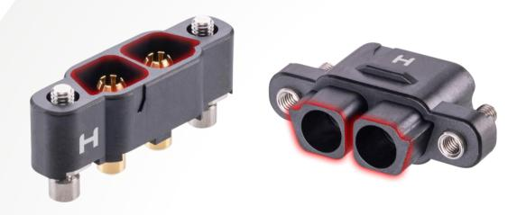
Contacts on the Kona range are all individually shrouded, with a recessed design. This helps prevent accidental touch of contacts by locating the contact end below the housing face. The contacts are also better protected against incidental damage from physical knocks or mis-mating.
