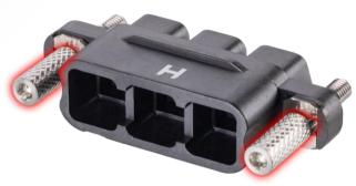
All Kona connectors are fitted with screw-lock fixings, to achieve the maximum vibration and shock specifications. They are also mate-before-lock, so connectors are easier and faster to mate before the screws are engaged and screwed together.
